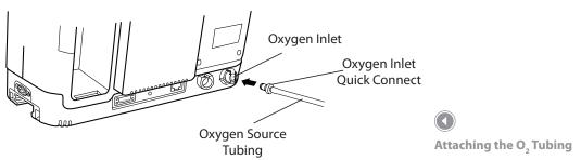
2. Make sure you press the Oxygen Inlet Quick Connect firmly into the inlet. You should hear a click, and the latch at the top of the inlet will pop up.
